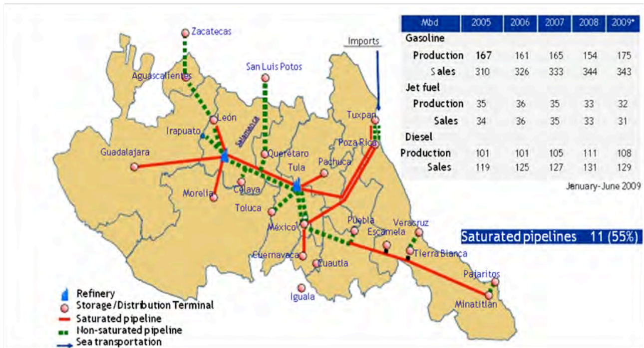
Figure 8.12: Pipeline Network in Central Zone
