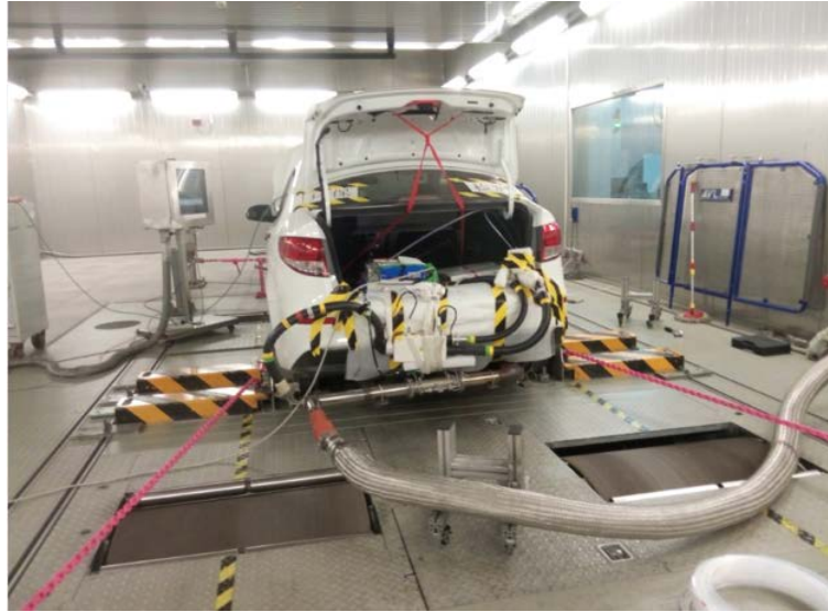
Figure 6 PEMS verification on chassis dynamometer
