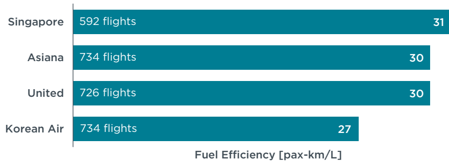
Figure 5. Fuel efficiency for airlines serving San Francisco-Seoul route
