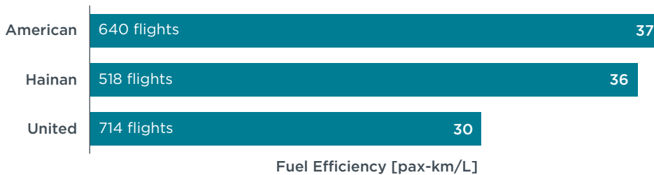
Figure 8. Fuel efficiency for airlines serving Chicago-Beijing route
